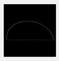
Arches with integrated bottom yard boarder 53 pixels w/ 159 total LEDs on the Arch 32 pixels w/ 96 total LEDs on the bottom section Link to 3D Printed Arch Bases
