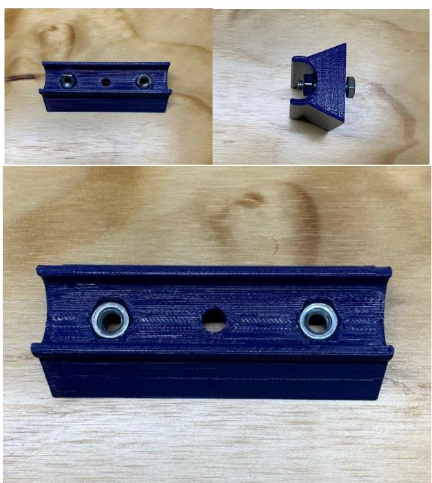
Flip the piece over and repeat the process for the center nut. In order not to damage the curvature of the EMT side, I thread the bolt past the nut about  $\frac{1}{4}$ ", align the nut with the opening and use a hammer on the bolt to gently tap the nut flush with the surface.
