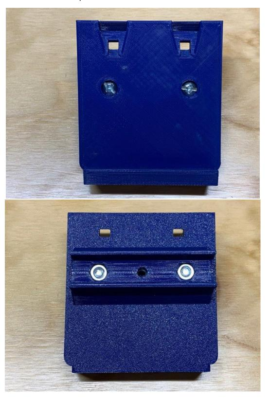
The recessed center nut is used to secure the EMT conduit directly to the mount using a 1  $\frac{1}{4}$ " screw or bolt if desired. Drill a  $\frac{1}{4}$ " hole in the EMT where it aligns to the mount and tighten the screw or bolt to secure. With the EMT conduit in place, the 1  $\frac{1}{4}$ " length will end flush with the back of the nut and not penetrate the mounting plate.
