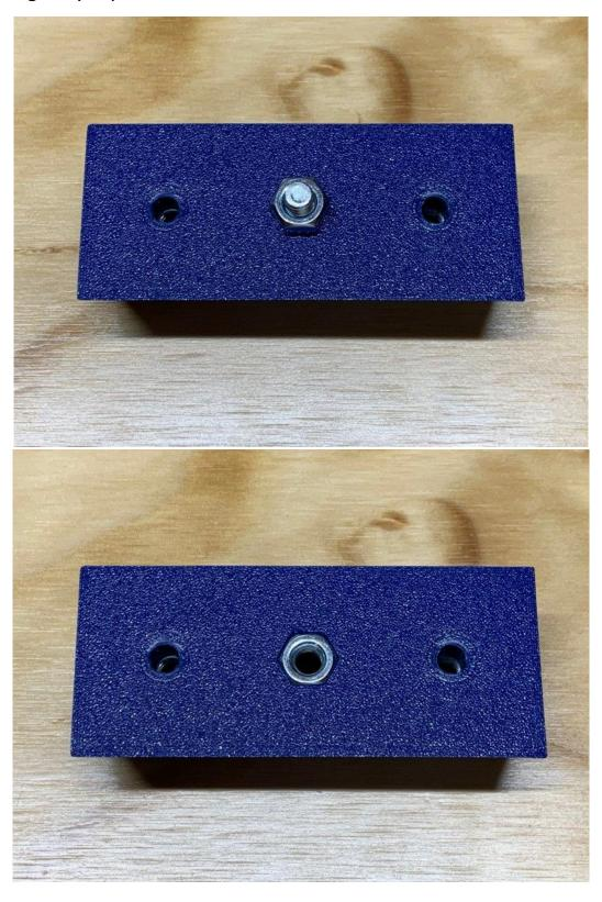
Lastly using the ¾" screws, screw the EMT mounting piece to the plate. The screws should recess below the surface with nothing protruding into the EMT conduit's path.
