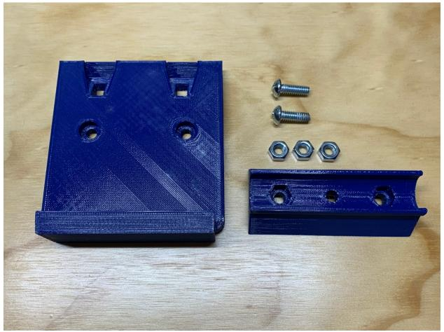
Insert hex nuts into the EMT mounting piece. The fit is tight so using a bolt or screw to pull the nut into position from the opposite side is required. I find using a 1" bolt works the best since I can use a ratchet to tighten. Make sure you align the nut with the opening when tightening down so that it fits into the hole cleanly.
