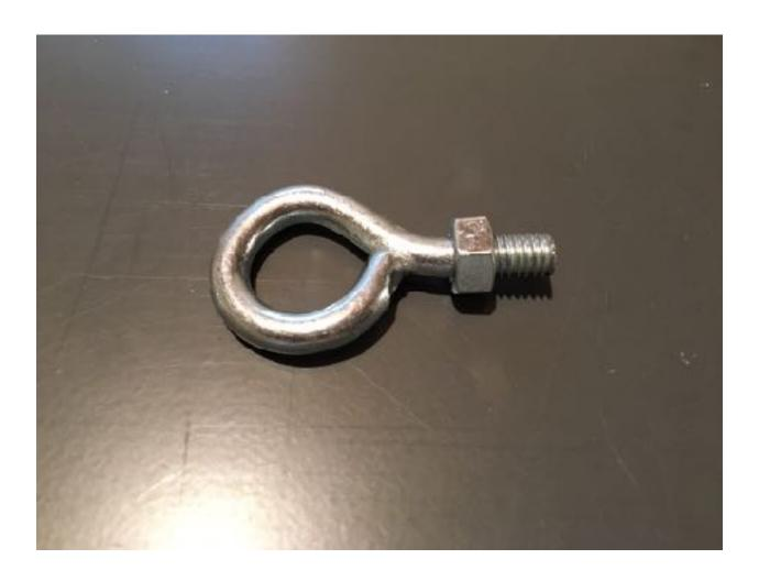
Assemble the 5/16" Eye Bolt into the Muffler Clamp as shown and tighten. I recommend using thread locker during assembly of all parts.
