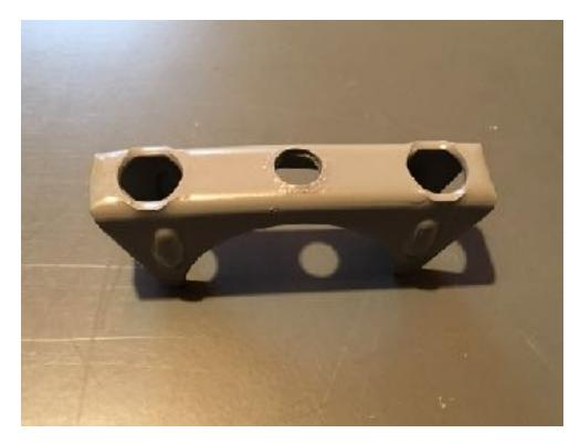
Drill a 5/16" into the center of one of the Muffler Clamps.
