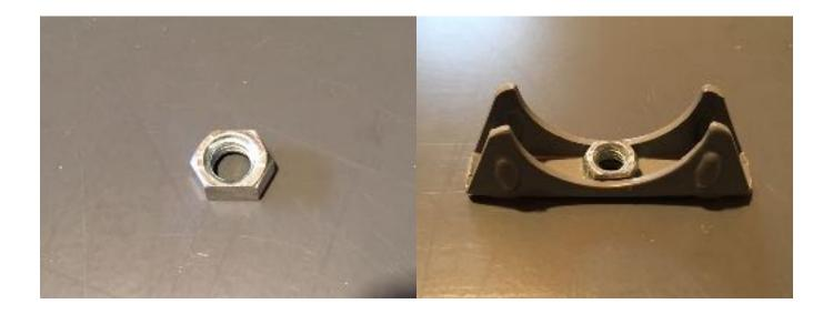
Next further grind the 5/16" Nut to match the curvature of the Muffler Clamp. A Dremel tool with a rough grit sanding disk work well for this.
