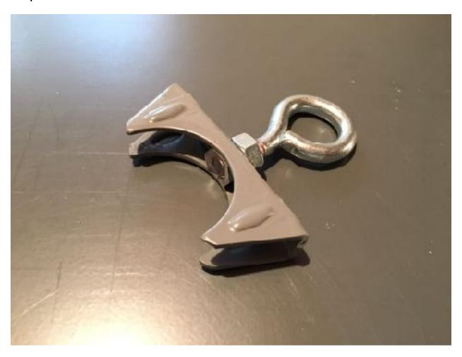
On the 3/8" Eye Bolts place the nut at the top of the threads, then insert the 5/16" washer and slide the other Muffler Clamp into position.
